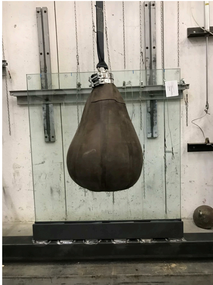
Photograph of the item after impact in the center of the glass
